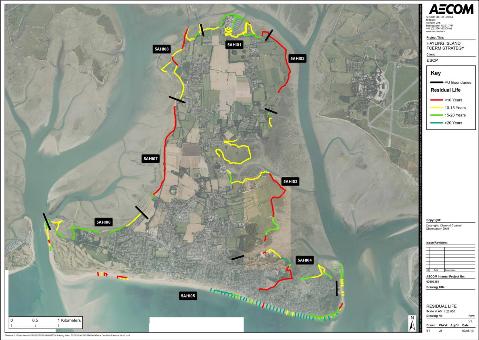
Figure 6-1. Estimated residual life of the defences
