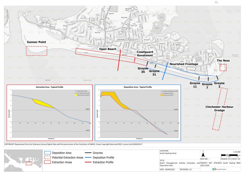
Figure 5.1: Extraction & deposition along the South Hayling frontage
