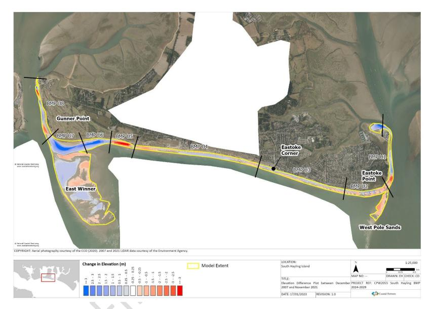
Figure 2.13: LiDAR difference plot showing beach change between 2007-2021, including changes over the East Winner and West Pole Sands ebb tidal deltas
