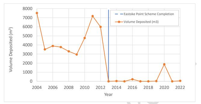
Figure 3.4: Volume of shingle deposited between groynes 6-11 (2004-2022)
