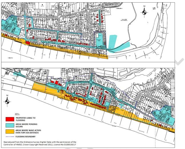
Figure 1.12: Areas liable to flood due to wave overtopping prior to the 1985 beach replenishment scheme, based on HBC drawing no. 1007/358, March 1997
