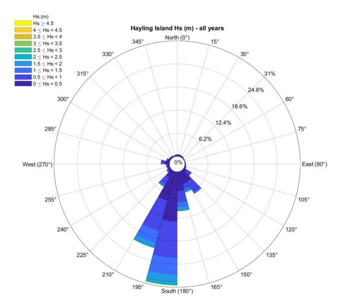
Figure 2.3: Significant wave height direction, Hayling wave buoy (2003-2022) (Ref 2.11)
