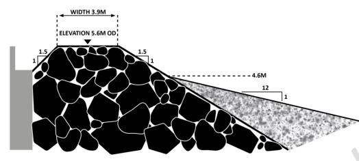
Figure 3.8: Eastoke Point Scheme design profile
