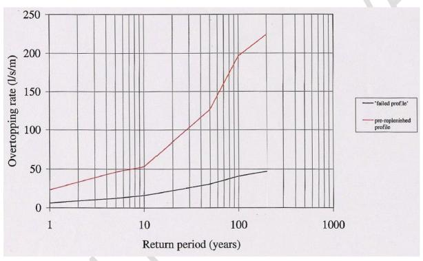
Figure 3.6: Overtopping rate of failed and pre-nourishment profile
