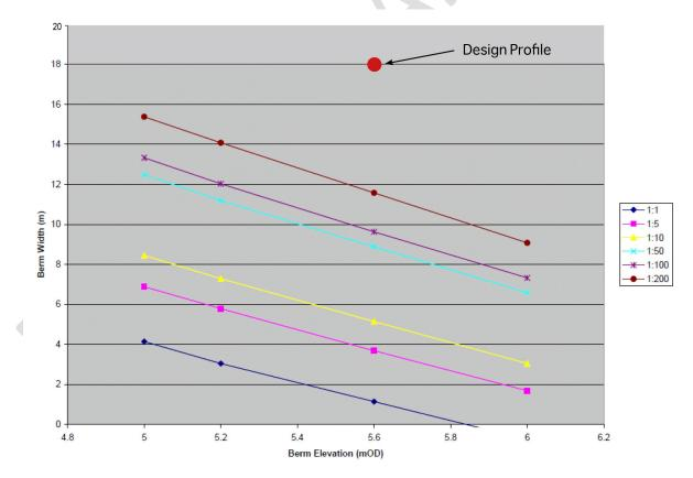
Figure 3.5: Beach design profile parameters for varying overtopping standards of protection
