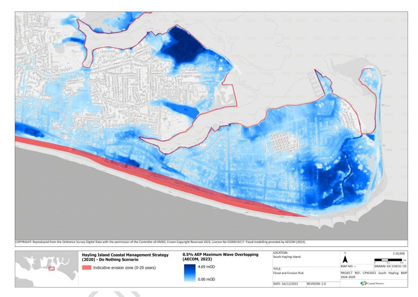
Figure 1.2: The 0.5% AEP flood risk zone and 20-year erosion zone under a "Do Nothing" scenario.
