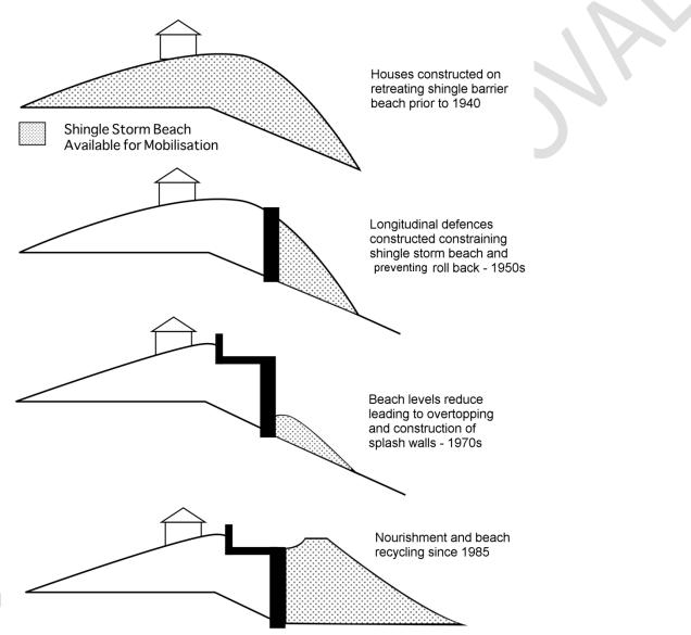
Figure 1.10: Process of beach constraint through construction of shore parallel defences at Eastoke, Hayling Island (Ref 1.7)
