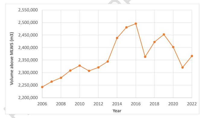
Figure 2.14: Total beach volume change along the South Hayling frontage (for a breakdown of separate BMP units refer to Figure 2.15)
