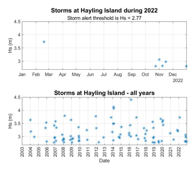
Figure 2.4: Incidence of storms since 2003 where Hs > 2.8m (the Storm Alert Threshold for Hayling Island is based on the 0.25 year return period for significant wave height which is 2.8m) (Ref 2.11)
