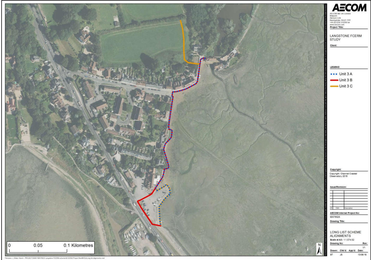
Figure 5-1: Potential defence alignments for Unit 3
