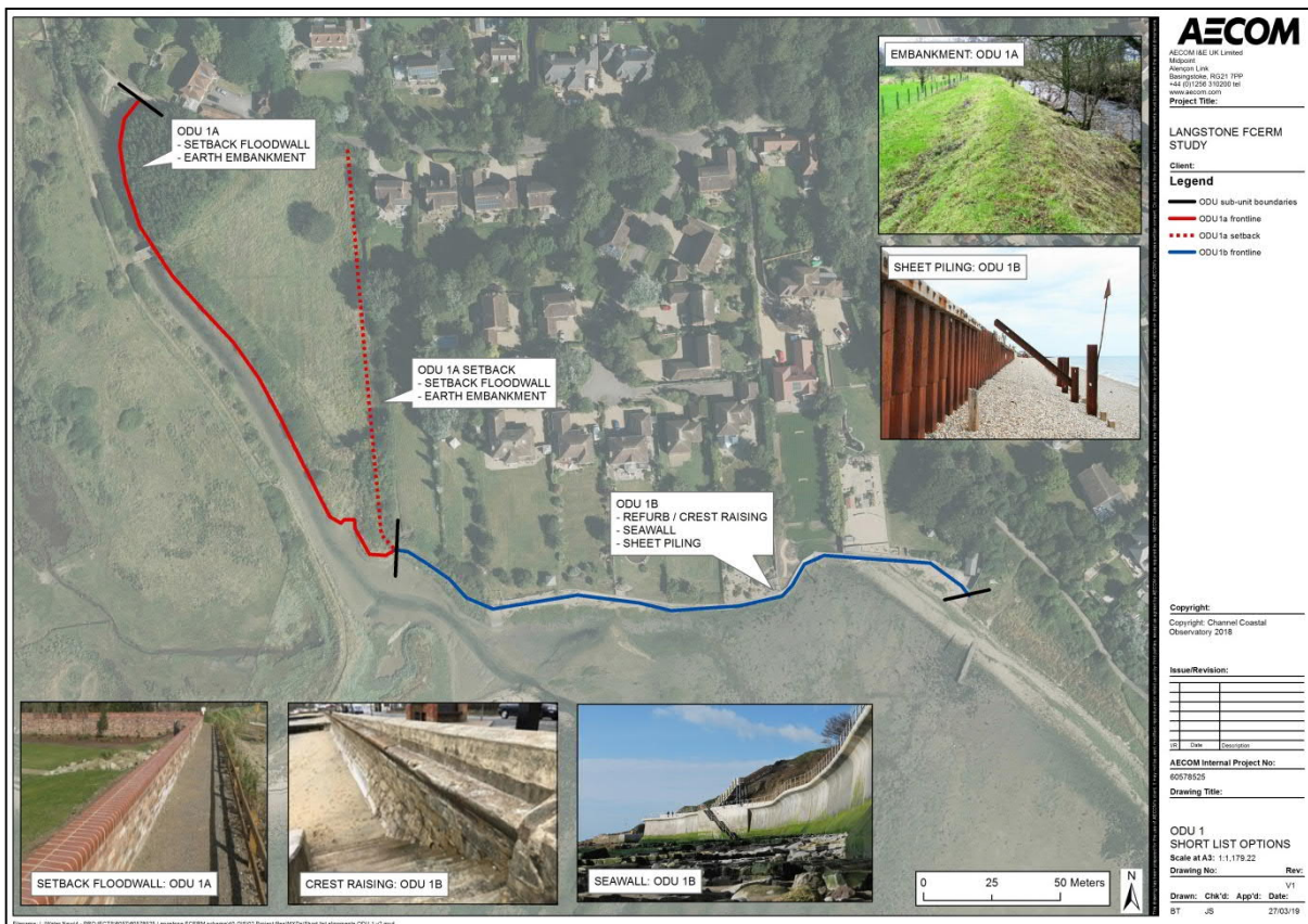
Figure 2-2: ODU 1 short list defence measures and alignments
