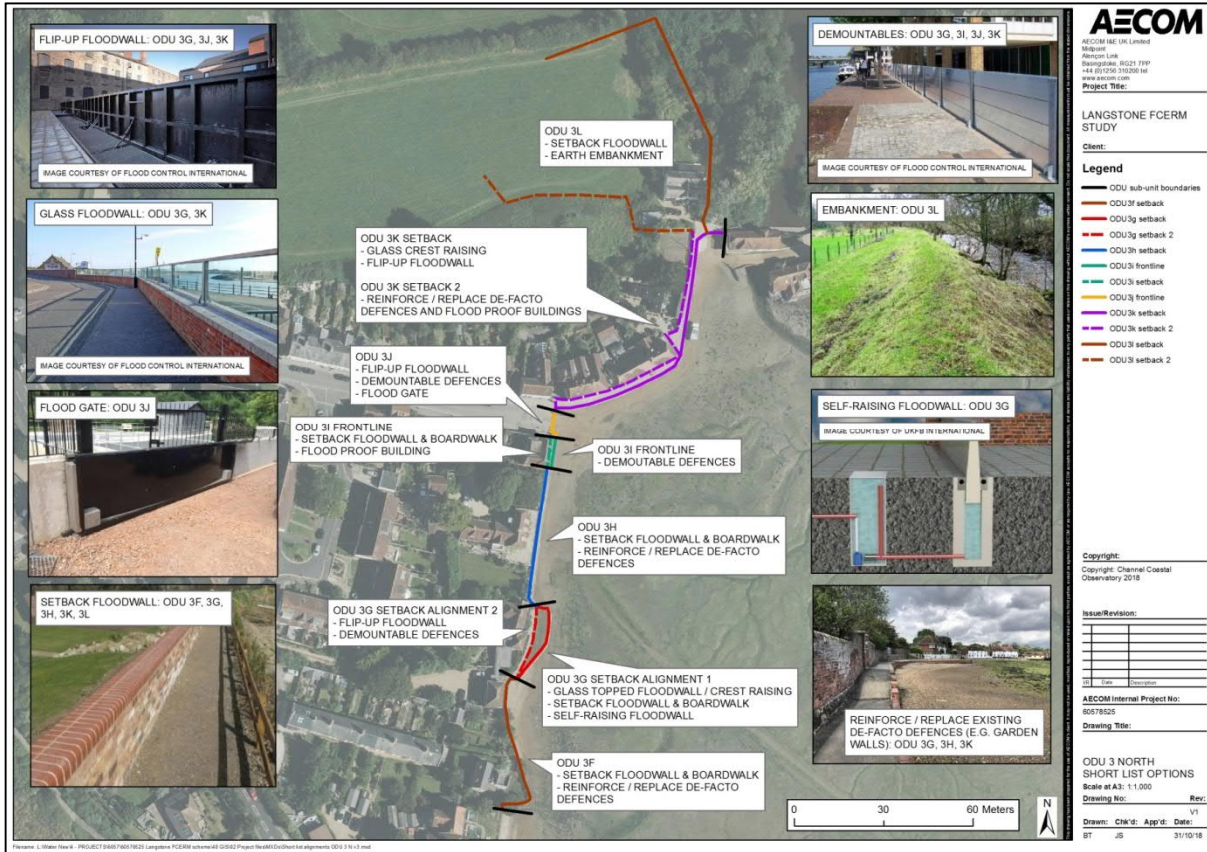
Figure 2-5: Short list defence options and alignments in ODU 3 (north section)
