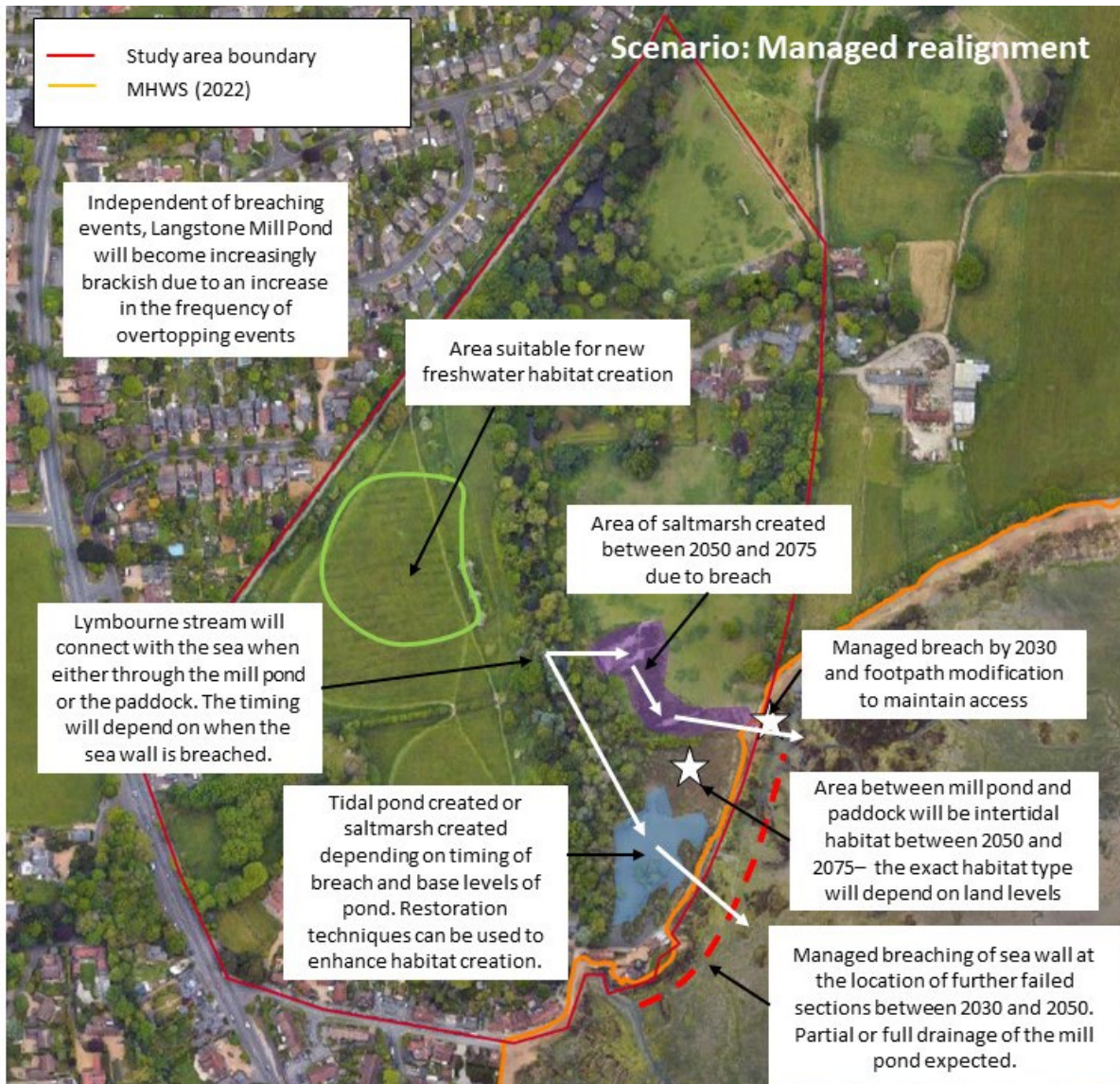
Figure 31: Proposed section of the sea wall to be breached – dashed red line.
