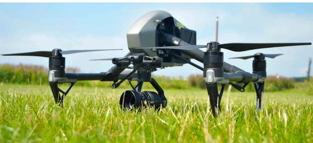
Each drone offers advantages in different environments and the team rotates them when required. The Ebee X is fantastic for surveying vast areas, providing adequate space for take-off and landing are available. Due to its vertical climb, the DJI Quadcopter is essential for areas where access and space are more difficult. It is also very efficient for localised surveying and shoots excellent 4K images.
