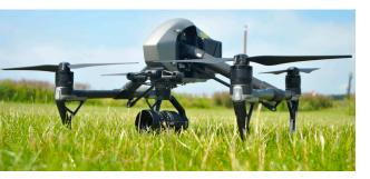
Each drone offers advantages in different environments and the team rotates them when required. The Ebee X is fantastic for surveying vast areas, providing adequate space for take-off and landing are available. Due to its vertical climb, the DJI Quadcopter is essential for areas where access and space are more difficult. It is also very efficient for localised surveying and shoots excellent 4K images. By using drones,
