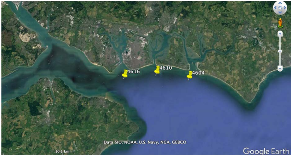
Figure 2.2 Extreme water level grid points 4616, 4610 and 4604 from the Extreme Sea Level study within the EA’s Coastal Flood Boundary Conditions for UK Mainland and Islands guidance (Ref 2.5)
