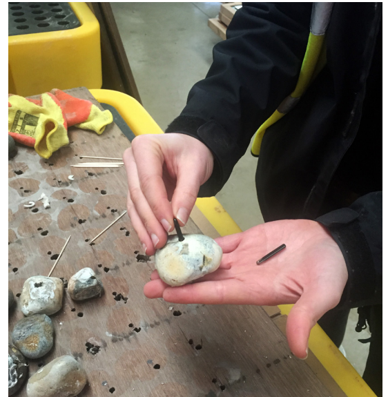
Figure 2: RFID tags sealed into local pebbles
